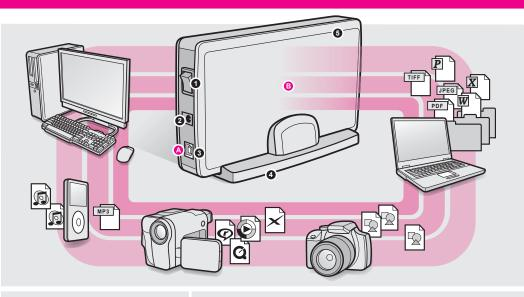
1 Power switch 4 Enclosure stand 2 Power port 6 Metal casing 3 USB port
